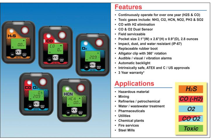
The 04 Series single gas monitor is designed to operate for many years with field replaceable sensors and filters. The 04 Series can be operated continuously for up to 9,000 hours on (2) AAA size alkaline batteries (depending on model). The 04 Series has 3 preset alarms that are user adjustable. Each version is also equipped with visual, audible, and vibration alarms as standard.
