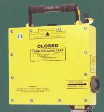
Triple-function portable gauging tape.
