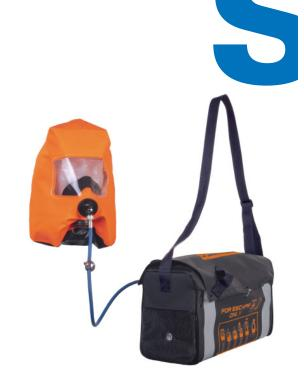
SK 1203 is designed to grant to the user a constant flow of air to escape from the dangerous surrounding, at the end of the air reserve a special valve opens and allows to breath ambient air that at that point shall be free of contaminant.
