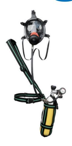
The supporting harnesses can be regulated and they allow to put the cylinder in the most comfortable position on the operator side or front allowing him to move even in narrow places. The pressure reducer keeps the outlet pressure constant throughout the emptying of the cylinder and is connected to an easy to read phosphorescent gauge. The steel or composite cylinder has a capacity of 3 liters with a pressure of 300 bar and is fitted with a valve according to EN 144.
