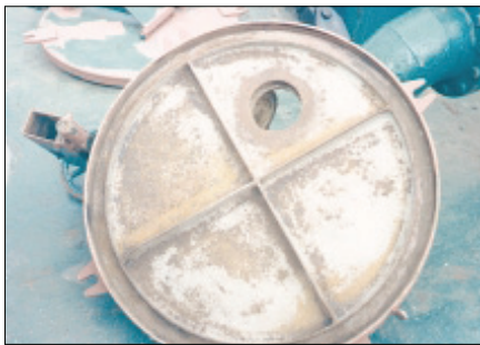
Step 1 Preparation of the surface can be made also by wire brushing. It is advisable ST-2 Standard preparation. If present remove rust chips, millscale, blisters, grease etc.
