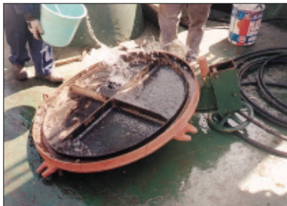
Step 2 Flushing with fresh water to remove atmospheric salts.
